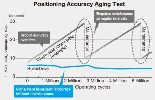
The RollerDrive graph is based on internal testing. (Center distance of test unit: 170)
