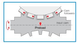
Multiple roller followers, come into contact from both sides (in pairs) without gaps to provide efficient rolling transmission without backlash.
