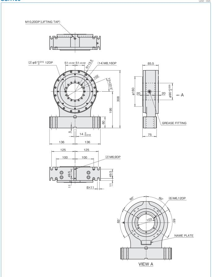
**SSR195-J** Unit: mm  $0.2^{-0}_{-0.2}$ 12×(φ9) P-6N (NBR-90)  $12 \times \phi 4$ M10,20DP(LIFTING TAP) (φ18) P-14N (FKM-90) OUTPUT SURFACE 222 212.5  $(2)\phi 8^{+0.015}_{0}$  12DP 51±0.02 51±0.02 (14)M8,16DP 85.5 105.7  $\phi$ 160 φ91 308 11 92 96 9 GREASE FITTING 2 14-0.018 75 136 136 125 125 (2)M6,9DP 100 100 49.5 0 0 MA\_⊚ 0 8×11 PORT 1~12 ROTARY JOINT 2×12×Rc1/8 CENTER PORT ROTARY JOINT Rc1/4 NAME PLATE VIEW A
