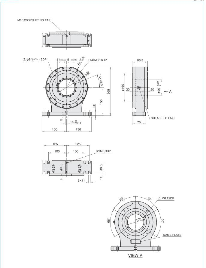
**SSR155-J** Unit: mm 0.2 -0.2 P-6N (NBR-90)  $12\times\phi4$ M10,20DP(LIFTING TAP) (φ18) P-14N (FKM-90) OUTPUT SURFACE 222 212.5  $(2) \phi 8^{+0.015}_{0} 12DP$ (14)M8,16DP 51 ±0.02 51 ±0.02 85.5 105.7 15×22.5° φ113.5  $\phi$ 160 φ91. 268 11 155 **-** Α 96 GREASE FITTING 2 14-0.018 75 136 136 125 125 (2)M6,9DP 100 100 49.5 49.5 0 0 8×11 PORT 1~12 ROTARY JOINT CENTER PORT ROTARY JOINT Rc1/4 2×12×Rc1/8 5 NAME PLATE VIEW A
